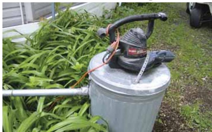
Leaf blower attaches to lid of garbage can outside house. Metal pipe runs into basement and hooks up to a vacuum cleaner hose, which sucks ashes from stove’s firepot.
