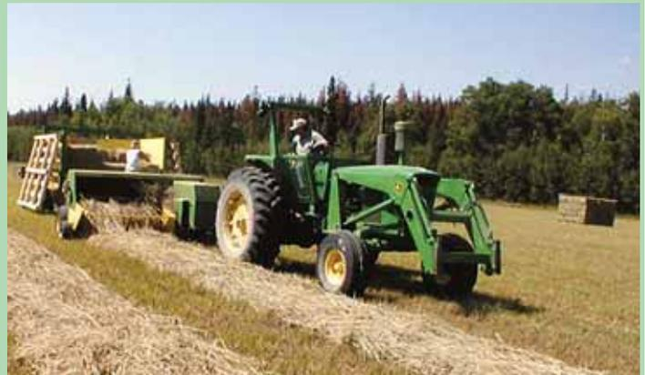
Keddie's "pallet" cart pulls directly behind baler. Extra pallets store on sides of cart. It leaves neat stacks of bales in the field, as shown at right in photo.
