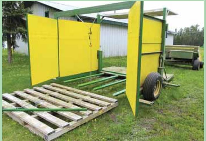
Pallet slips over 4 long forks to form cart's floor. After bales are loaded, Keddie lowers forks to ground, then drives forward to leave pallet in the field.
