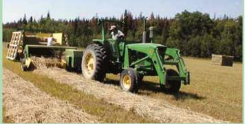
Keddie's "pallet" cart pulls directly behind baler. Extra pallets store on sides of cart. It leaves neat stacks of bales in the field, as shown at right in photo.
