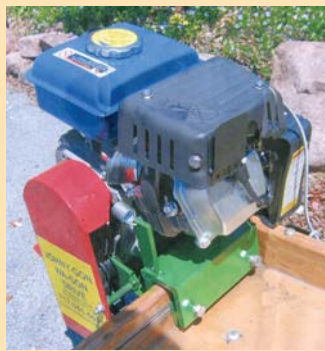
A 2 1/2 hp Greyhound engine clamps onto back of wagon and is used to friction-drive one of wagon's rear wheels.
