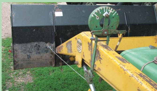
Attached to loader arm, homemade tilt gauge lets Clifford Tonsfeldt see the bucket angle at a glance when digging or picking up material.
