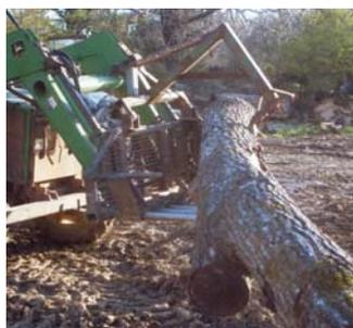
Bucket can be used together with a hydraulic-operated, L-shaped "squeezer clamp", which pins onto angle iron brackets welded across top of bucket.
