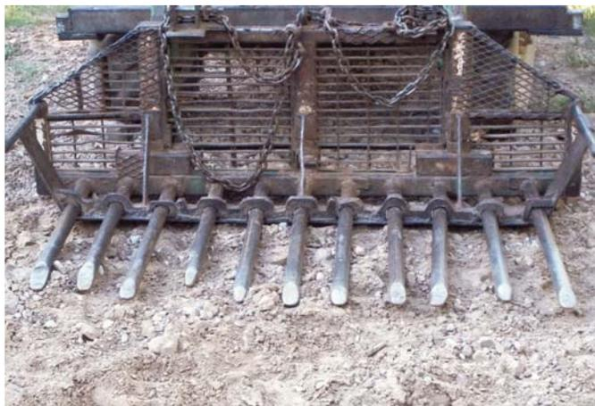
A series of 3-ft. long forks fit into slots on front of bucket. Metal grating on back makes it easy to see what's happening.
