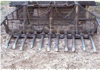
A series of 3-ft. long forks fit into slots on front of bucket. Metal grating on back makes it easy to see what's happening.
