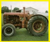
and installed it in a 1938 W30 model The engine fit almost perfectly. I had to extend the engine mounts and move the exhaust pipe from the left to the right side and also move the air breather back used the tractor to operate a threshing machine and sawmill at the LA Vintage Machinery Show in Lacombe, Alberta. I also tried it out at a local demonstration
