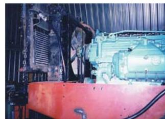
Ed Sokalski spent less than \$2,000 to install a 6-71 "Screaming Jimmy" two-stroke diesel engine in his International 4386 4-WD tractor. "It has more torque and runs better than the original engine," Sokalski says.
