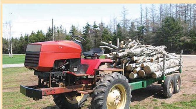
Leo Gallant built this strange-looking tractor by combining parts from an old 1950's Cockshutt tractor with a garden tractor.
