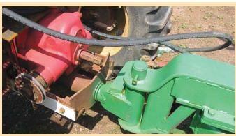
Tractor's "articulated" steering system uses a hydraulic cylinder and hinge on the drawbar that mounts to a permanently attached trailer.
