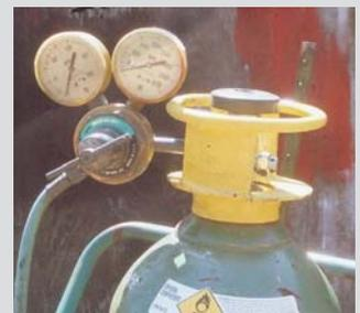
which screws onto the oxygen cylinder, is off a commercial storage cap - I simply cut the bottom off. The safety cap is designed so I still have full access to the cylinder's shutoff valve at the center top, and to a pair of gauges on one side.
