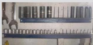
**Chuck Knipp, Palco, Kan.:** "I have a lot of sockets in my shop without cases and nowhere to put them. So I made a socket holder using a piece of 1 1/2-in. angle iron mounted to the wall. I spaced the sockets out on the bar and then marked each location with chalk. Then I ground down the points on some nails and tack-welded them to the bar. After a little paint, I had a cheap, durable socket holder."
