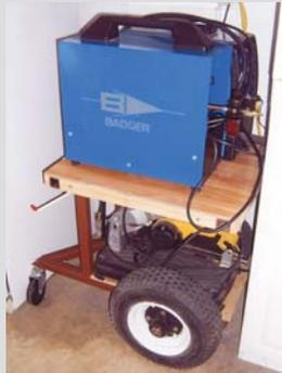
**Warren Lauppe, Merced, Calif.:** "I made a small cart to carry my welder, cut-off saw and air compressor. It's designed to make a tight turn to fit into a small space in my garage. And it has large tires so it will move easily over uneven surfaces. The top shelf is cantilevered over the back without rear posts so it's easy to remove the cutoff saw from the bottom when needed."
