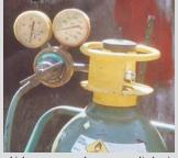
which screws onto the oxygen cylinder, is off a commercial storage cap - I simply cut the bottom off. The safety cap is designed so I still have full access to the cylinder's shutoff valve at the center top, and to a pair of gauges on one side.
