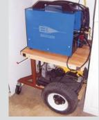
Warren Lauppe, Merced, Calif.: "I made a small cart to carry my welder, cut-off saw and air compressor. It's designed to make a tight turn to fit into a small space in my garage. And it has large tires so it will move easily over uneven surfaces. The top shelf is cantilevered over the back without rear posts so it's easy to remove the cutoff saw from the bottom when needed."
