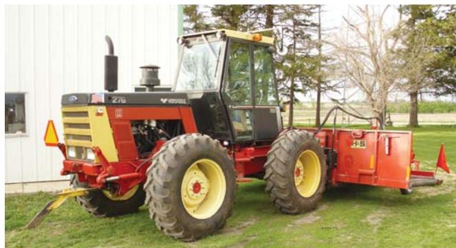
Virgil Pook and son Travis reversed the mounting brackets and drive system on their pull-type windrow merger so they could push it rather than pull it.
