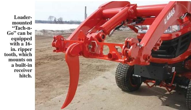
Loader-mounted “Tach-n-Go” can be equipped with a 16-in. ripper tooth, which mounts on a built-in receiver hitch.
