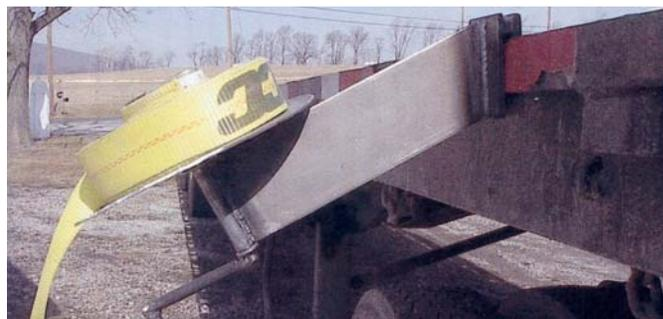
Hand-operated “ratchet strap winder” is designed to quickly roll up round bale straps. It can be moved anywhere on trailer.
