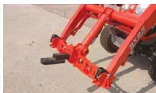
Receiver hitch (top) can be used with trailers. Two-component locking mechanism consists of a bolt and compression spring.
