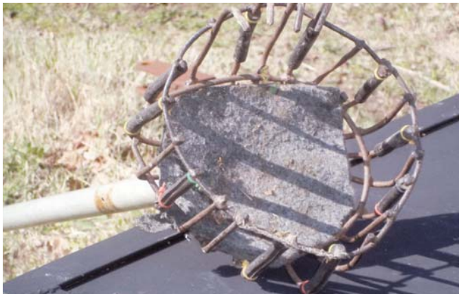
Fruit picker’s aluminum handle supports an 8-in. dia. wire basket. Four curved metal fingers on one side of basket bend inward at 90 degree angle to pull in fruit.
