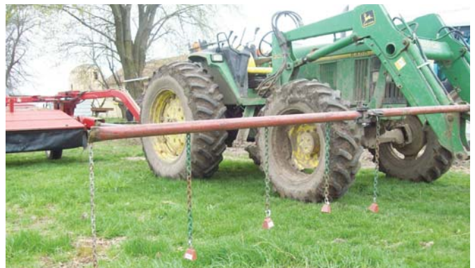
Loader-mounted pipe has a series of chains hanging down from it. Cow bells are welded to bottom of each chain.
