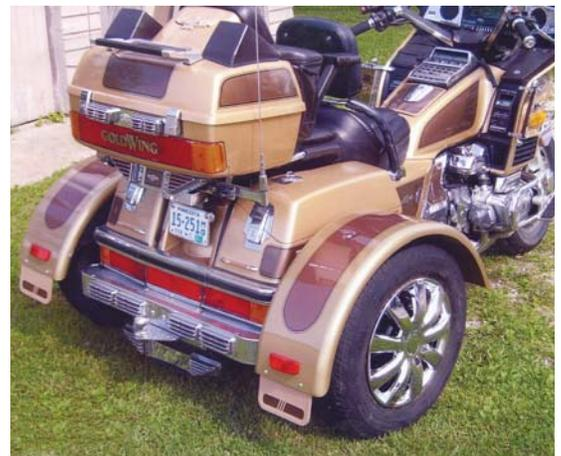
Loren Smith converted his 1985 Honda Goldwing motorcycle to this 3-wheeler, adding an axle and a pair of 14-in. wheels off an old mini van on back.
