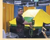
Flexible combine hopper cover comes with an electric actuator that's remotecontrolled from the cab.
