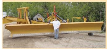
Heavy duty plow makes 32-ft. wide drainage ditches in a single pass.
