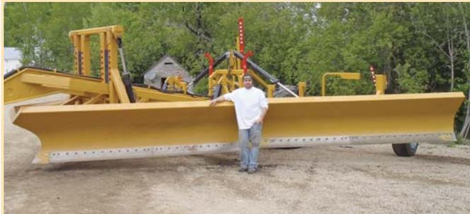
Heavy duty plow makes 32-ft. wide drainage ditches in a single pass.
