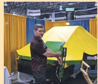
Flexible combine hopper cover comes with an electric actuator that's remote-controlled from the cab.
