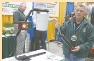
Wireless probe hangs vertically from auger and signals when bin is full.
