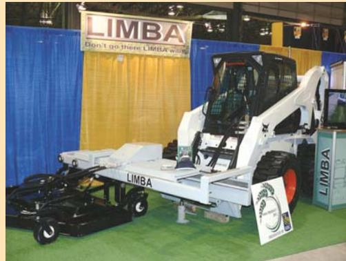
Side-shift front toolbar lets you shift a rototiller, mower or other hydraulic-powered implement up to 6 ft. to either side of tractor.
