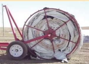
Ground-driven unit rolls up empty silage bags into a tight coil around a cone-shaped spool.
