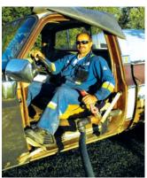
Belanger removed the driver's side door from his pickup, allowing him to water trees as he drives. Outlet hose is plumbed into a 350-gal. tank on back of pickup.
