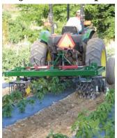
Each pair of tillage gangs, both front and back, are positioned to either side of row. Gang pitch can be adjusted up to 25 degrees.
