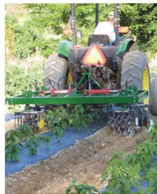
Each pair of tillage gangs, both front and back, are positioned to either side of row. Gang pitch can be adjusted up to 25 degrees.
