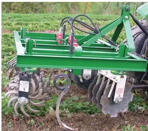
Cultivator has rolling coulters on front and 5-tine Lilliston spider wheels on back. S-tine shanks in the middle break up tractor wheel tracks.
