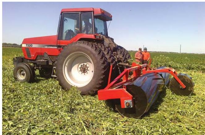
Roller’s chevron pattern grips the ground to reduce bouncing. Each roller has 23 angle irons mounted at 8-in. intervals, with the edges welded to the roller.
