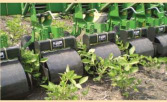
Each roller is 16 in. dia. and has a clamp-on toolbar mounting bracket on front.
