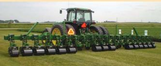
Culti-Rollers were field tested last spring on this 18-row Deere cultivator. Rollers can be filled with water or sand to add weight.
