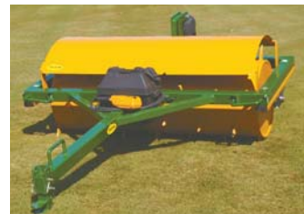
To mount different implements, a steel frame can be moved like a wheelbarrow and rolled over top of implement.
