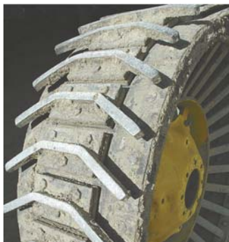
New kind of steel wheel uses a base of rubber belting secured to steel bands over wheel spokes.
