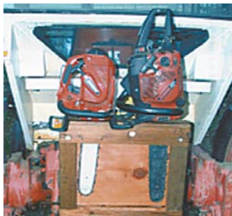
Carrier holds two chainsaws and includes a tiltable metal tray that can be used to hold log chains or other supplies.
