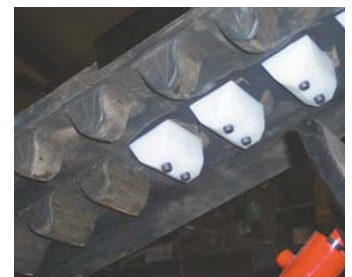
Bolt-on replacement lugs can be installed with the track on or off.
