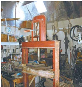
Don Ramberg built this 6½-ft. tall, 12-ton press more than 30 years ago and says it can still handle any job he throws at it.
