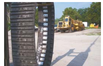
When track becomes unusable, you can remove the lugs and use them on another track.
