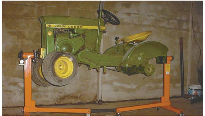
Wheeled garden tractor “rotisserie” keeps tractor about 30 in. off the ground.
