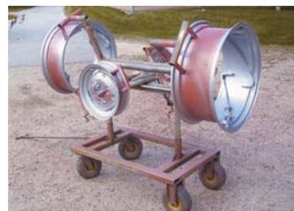
**This rack was made to paint wheel rims. “It holds the wheel inside the rim so I can spin the rim around as needed to paint,” says Hinckley.**
