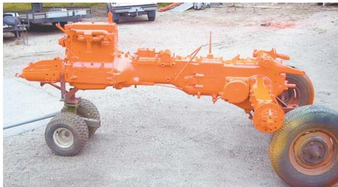
**Bill Hinckley’s home-built rolling stands make it easy to move tractor parts and frames whenever he needs to paint or sandblast. Photo shows a stand fitted with a Case tractor frame for doing restoration work.**
