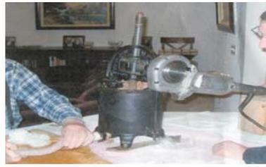
Powered pipe threader drives hand-cranked sausage stuffer.
