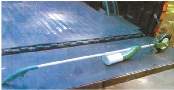
To use "chemical edger", pull a trigger on handle and start rolling the wheel. Chemical flows through hose down to top of wheel.
