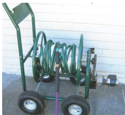
Hall's 4-wheeled steel hose reel is chain-driven by add-on gear reduction motor.
