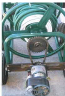
A sprocket mounts in place of reel's original crank handle.
