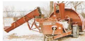
He used a Gehl 135 hammer mill for the base and mounted a bagger funnel top on the hammer mill's frame.
