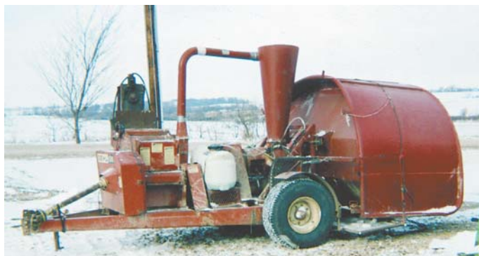
Custom silage bagger Marvin Martin built his own machine to bag high moisture corn.
