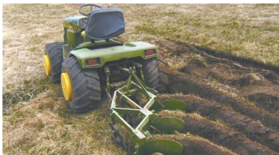
Glenn Peterson built this 4-WD, articulated, 25 hp garden tractor, adding 250-lb. weights to each wheel.
