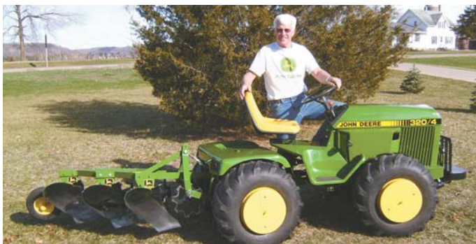
Glenn Peterson built this 4-WD, articulated, 25 hp garden tractor, adding 250-lb. weights to each wheel.
