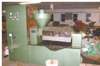
He runs the sunflowers through a Chinese oil press (left) and then runs the meal through a Chinese pelletizer.
