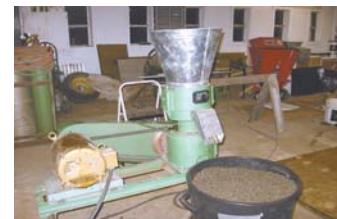
He runs the sunflowers through a Chinese oil press (left) and then runs the meal through a Chinese pelletizer.
