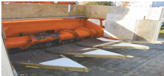
Roger Rainville made his own sunflower header by removing the reel from a Case 6660 combine and attaching homemade, V-shaped pans on the header.
