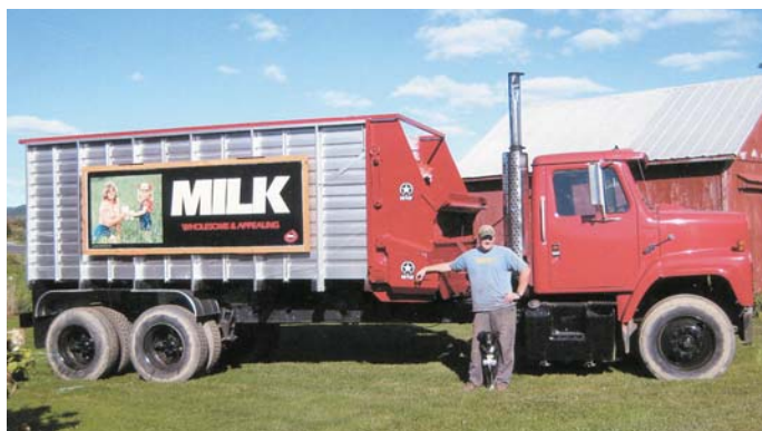
Using a neighbor's unit as a template, Wes Roberts converted a self-unloading wagon into this truck-mounted chopper box. Signs on side of box promote milk.
