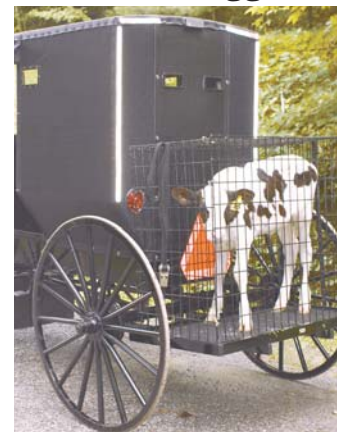
Add-on aluminum platform lets anyone with a one-horse buggy haul a calf or other cargo on back.
