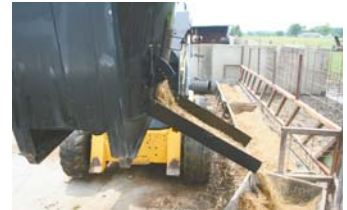
Three Indiana cattlemen came up with this skid loader-mounted tub mixer to feed wet distillers grain.
