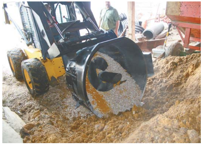
Three Indiana cattlemen came up with this skid loader-mounted tub mixer to feed wet distillers grain.
