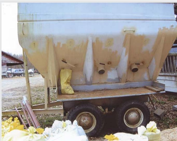
Modified fertilizer spreader is equipped with 3 ports on one side, allowing 3 workers at a time to fill sandbags.
