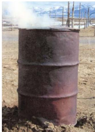
Barrel stands in a shallow hole. Note small opening, lower right, to let air into bottom of barrel.
