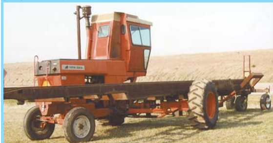
Axle on right side of combine was extended to make more room for trailer.
