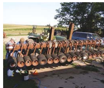
Prototype of new unit alternates steel drums with rubber tires.
