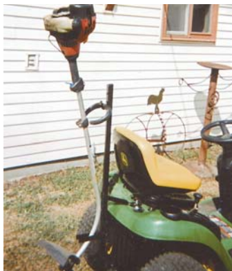
Homemade weed eater carrier mounts just behind lawn tractor's seat and is always there when Peters needs it.
