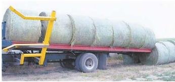
Lift arm mounts directly to truck frame and is made out of various sizes of tubing supported by 1-in, steel plate.
