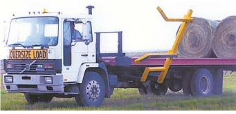
Modified 1991 Volvo cab-over truck can load and carry 14, 5-ft, bales. "I can load bales on-the-go, filling up in as little as 10 minutes," says inventor Dan Rosman.
