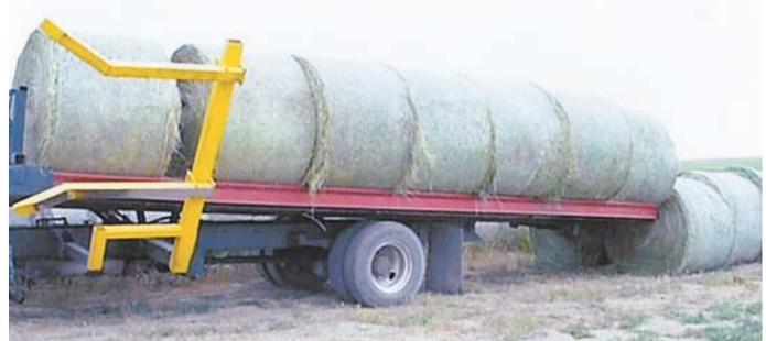
Lift arm mounts directly to truck frame and is made out of various sizes of tubing supported by 1-in. steel plate.
