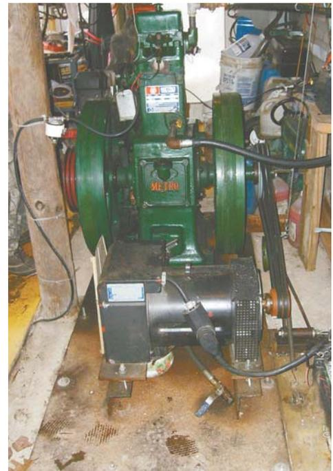
With add-on "cruise control", Lister engine-powered generator maintains steady power even when the generator (shown in the foreground) is under load.
