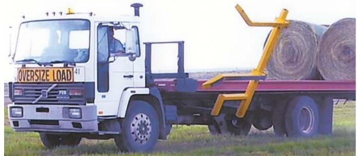
Modified 1991 Volvo cab-over truck can load and carry 14, 5-ft. bales. "I can load bales on-the-go, filling up in as little as 10 minutes," says inventor Dan Rosman.
