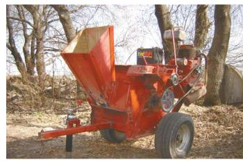
Portable wood chipper is built out of an old Gehl silage chopper. A Kohler 14 hp engine belt-drives the chopper's rotor.
