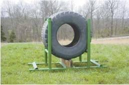
Big flotation tire sets in a cradle built out of oilfield pipe. It rides on runners made from 4 and 6-in. well casing.
