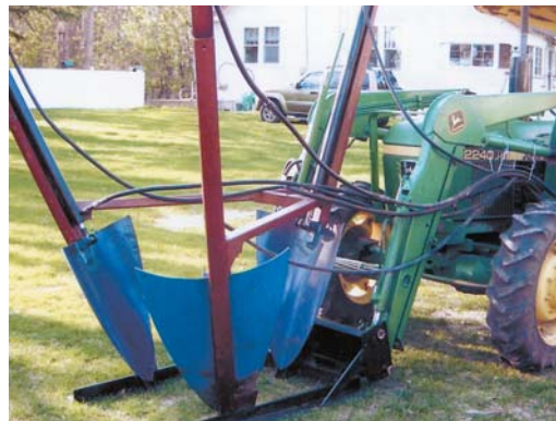
Duane Myklejord built this big 3-bladed tree spade to mount in place of the loader bucket on his Deere tractor. "I have a great view," he says.
