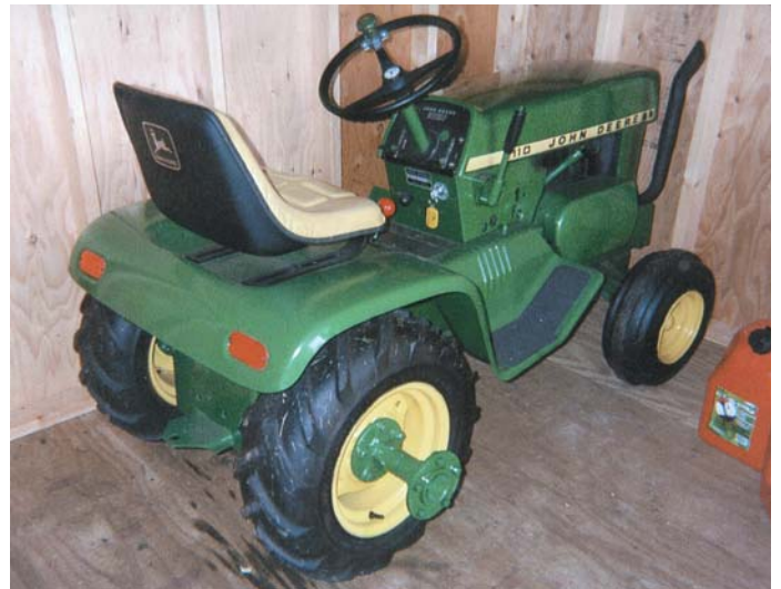
Dave Hartman used hubs salvaged from an older garden tractor to turn his Deere 110 garden tractor into a "dually".
