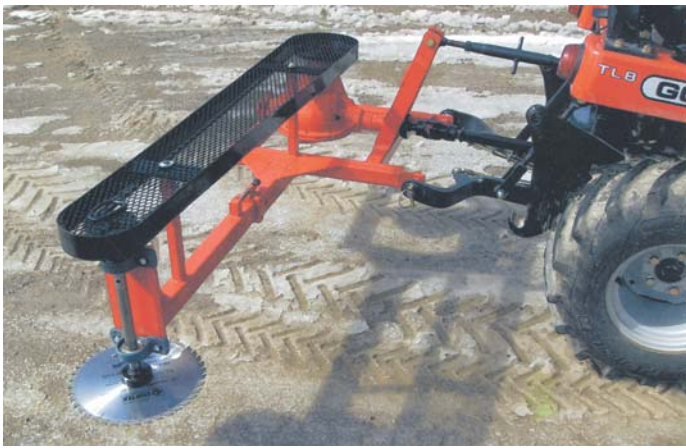
Pto-driven rotary brush cutter uses an automotive differential to belt-drive a 12-in., carbide-tipped table saw blade.
