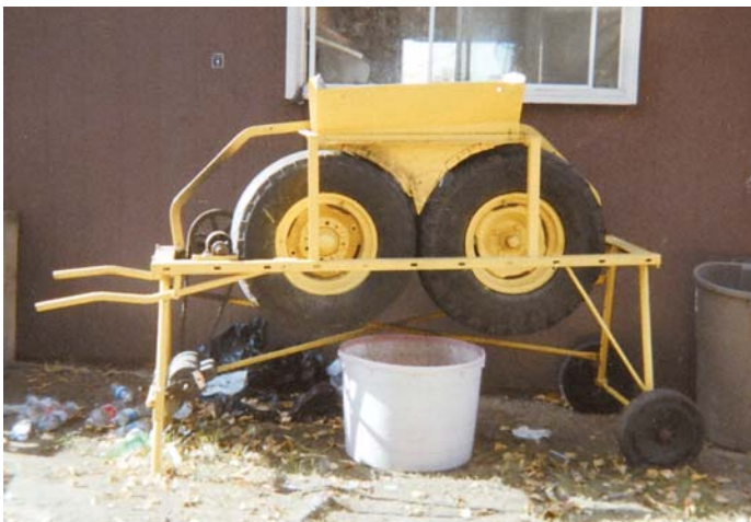
Powered can crusher is equipped with a couple of 15-in. high, 10-in. wide pickup tires, which run up against each other to crush cans.
