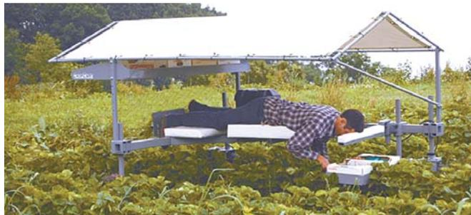
Battery-powered picking cart comes with a vinyl canopy that protects both the crop and the operator from sun or rain.
