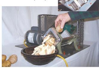
To make French fries, operator drops in one potato at a time and uses a foot pedal to activate the potato pusher.
