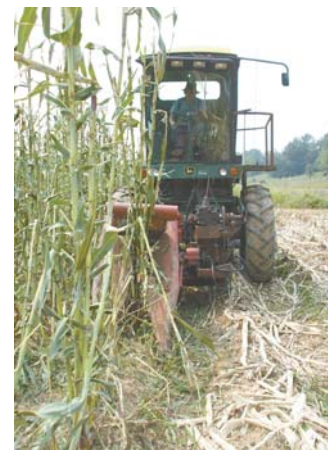
Stephens moved picker's cab back 31 in. to provide a better view of mill's rollers.
