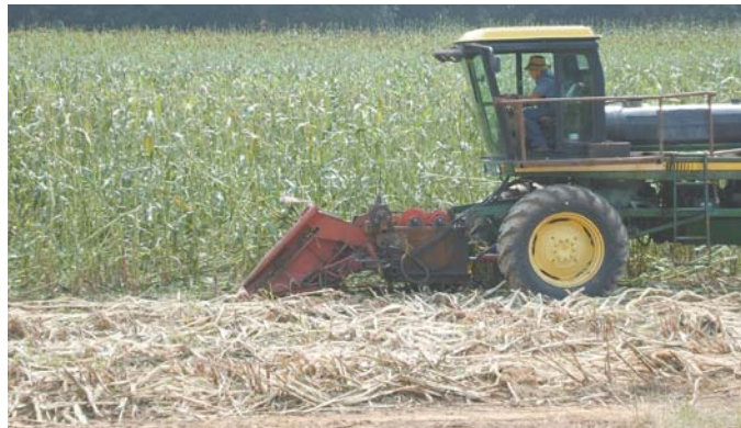
Mounted on an old cotton picker, sorghum harvester cuts sorghum stalks and feeds them through a mill.
