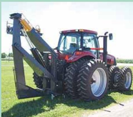
Interchangeable boots mount on quick-tach tile plow by simply pulling a single rod. Low angle knife is lined with stainless steel for less resistance as it opens the ground.
