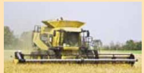
AWS air reels are available to fit all makes of combine headers. The curtain of air created by the manifold system across the front of the header provides an even flow of crop material into the combine with less damage.
