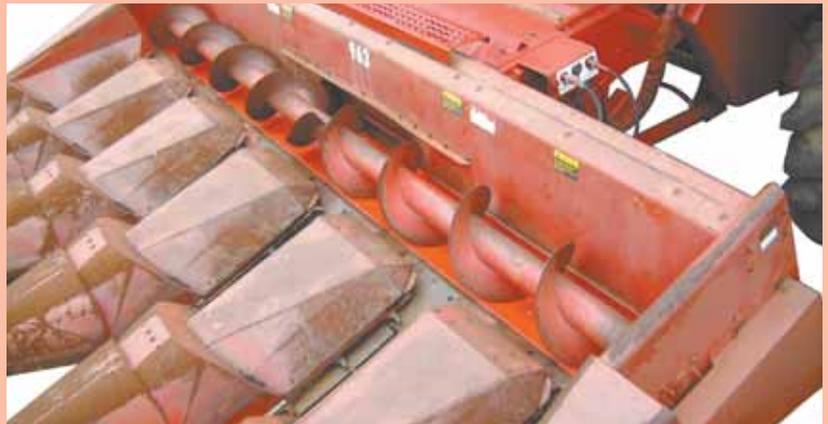
**Trough liner kit does not require removal of auger for installation. It's available for Deere, Case IH, and New Holland corn heads.**
