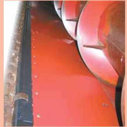
**Poly Feed Plate is reinforced with stainless steel at the center.**
