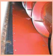
Poly Feed Plate is reinforced with stainless steel at the center.
