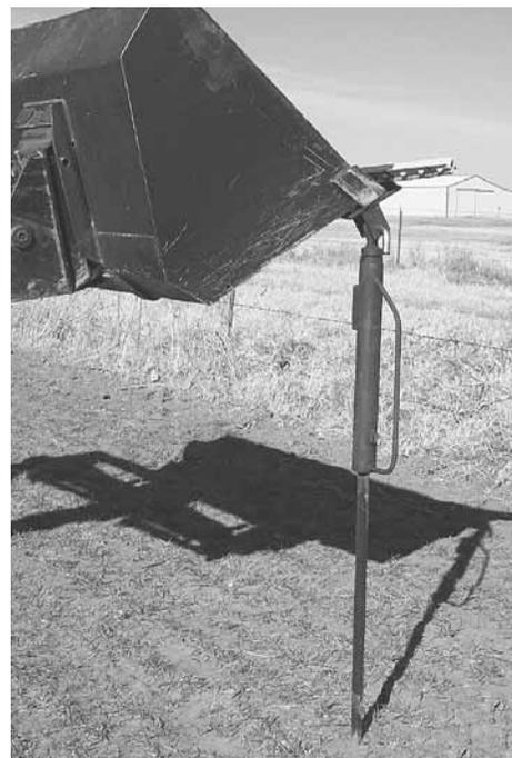
**Zweifel's T-post driver hangs from the front edge of loader bucket.**
