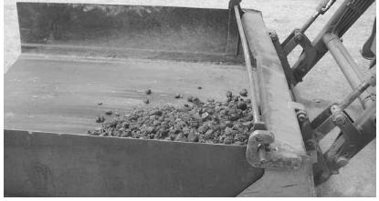
Steel basket hooks inside loader bucket to greatly increase its carrying capacity.
