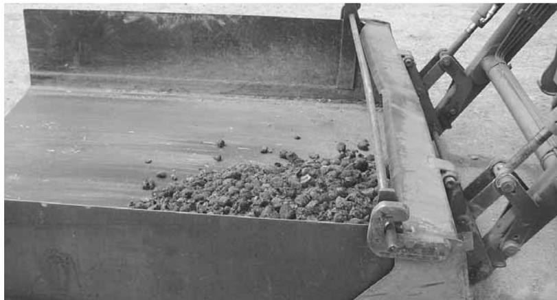
**Steel basket hooks inside loader bucket to greatly increase its carrying capacity.**
