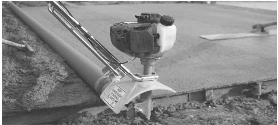
motor in a steel case making the power head more durable and less vulnerable to damage. Both the new Honda® gas powered motor and the new Rugged versions easily attach to the Classic Spin Screed® design which allows the user excellent versatility and convenience.
