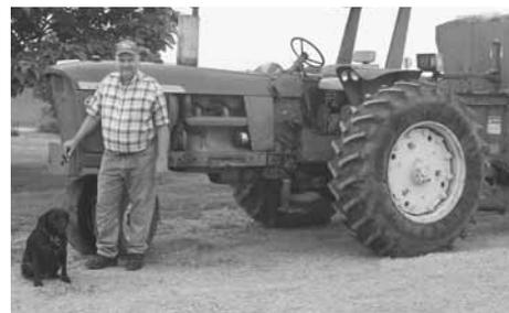
**Charles "Buddy" Myers is proud of his 1970 John Deere 4020 diesel tractor, which has more than 28,000 hours on it without ever overhauling the engine.**
