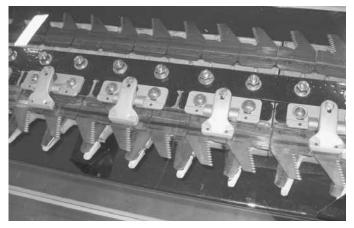
Sickle sections attach to roller chain that runs in a continuous loop.
